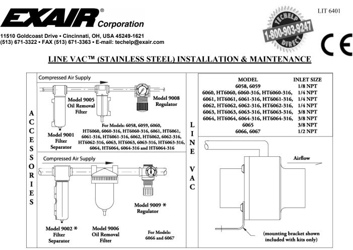
\* For Model 6065 - Use Model 9032 Filter Separator and Model 9033 Pressure Regulator
