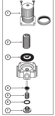
If leaks persist, remove bonnet, inspect diaphragm and diaphragm seat for wear or foreign materials.
