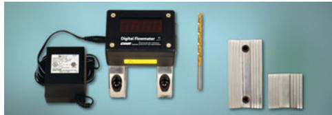
Each Digital Flowmeter includes an 18 VDC power supply, 3/16" drill bit, and hole locating fixture.
