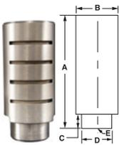
Heavy Duty Silencing Mufflers feature a corrosion-resistant aluminum outer shell with an internal stainless steel screen that protects valves and cylinders from contamination that could enter through the exhaust ports. This also keeps contaminants such as rust from being ejected at high speed from the exhaust port. The typical noise reduction is up to 14 dB.
