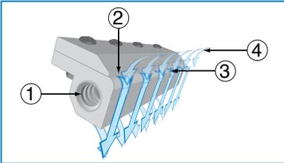
Compressed air flows through the inlet (1) into a plenum chamber. It is then throttled through a thin nozzle (2) extending the length of the Standard Air Knife. This primary airstream adheres to the coanda profile (3), which turns it 90° and directs the flow down the face of the unit. The primary stream immediately begins to entrain surrounding air (4), for an amplification ratio of 30:1 at 6" (152mm) away.
