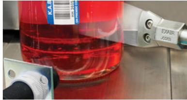
A stainless steel 1" Flat Super Air Nozzle removes condensate water from a label prior to scanning.
