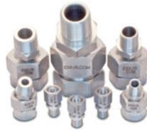
EXAIR's Swivel Fittings make it easy to adjust the position of the Air Nozzles, Air Jets, and Air Amplifiers. Swivel Fittings permit a movement of 25 degrees from the center axis for a total movement of 50 degrees. Type 303 and 316 stainless steel.
