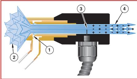
The Ion Air Gun incorporates a High Velocity Air Jet and electrically energized emitter point. A small amount of compressed air is injected into the air jet (1) inducing high volume flow of surrounding air (2) to pass through it.
