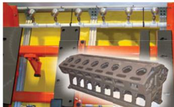
A series of Model 6042 2" (51mm) Adjustable Air Amplifiers blows coolant off 16 cylinder diesel engines.
