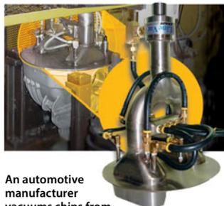
An automotive manufacturer vacuums chips from drive train differentials with a Model 150200 2" (51mm) Heavy Duty Line Vac.
