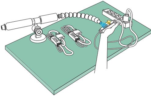
**The Problem:** A manufacturer of electrical heat tapes had a problem testing thermostats for accuracy. The heat tape is supposed to switch on when the outdoor temperature dips below 40°F to prevent pipes from freezing or ice from building up on a roof's edge. The liquid-tight thermostat of every tape had to be dipped into a bowl of ice water (thermometer checked at 36°F (2°C)) to make
