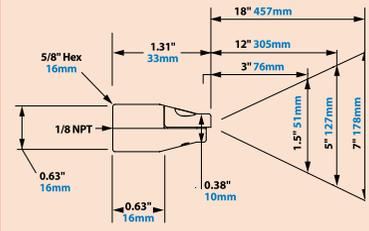
The Model HP11365S Shim Set for the 1" High Power Flat Super Air Nozzle includes a .020" (0.51mm) and .030" (0.76mm) thick shim. A .025" (0.64mm) shim is installed.
