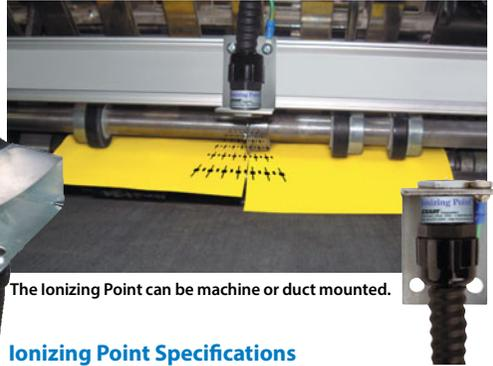
The Ionizing Point can be machine or duct mounted.
