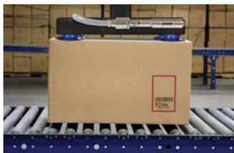
Compressed air use is minimized by selecting the exact vacuum level required to lift the heavy, porous cardboard cartons.
