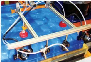
Model 7192 Ion Air Cannons provide static elimination in between solar panel lenses to assist separation of the lenses during production.
