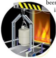
The timer was set to "on/off delay". The sensor was mounted at the oven exit (1 minute away from the blowoff station). When the sensor detected a tank, the timer turned the air on for one minute, just as the next tank reached the blowoff station.
