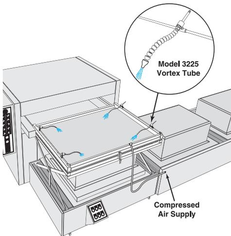
**The Problem:** A manufacturer of major appliances vacuum forms the plastic interior shell of refrigerators. The deep draw of the plastic and complex geometry left the four corners unacceptably thin. The corners
