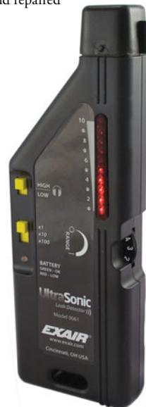
LED indicators on the Ultrasonic Leak Detector show the exact source of the leak or problem.
