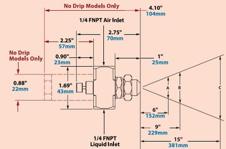
No Drip Only Dimensions in Red See page 69 for No Drip Atomizing Nozzles
