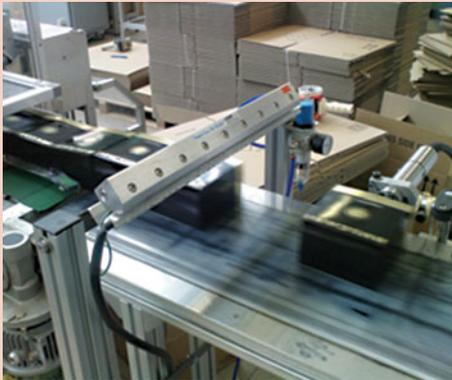
**The Problem:** A manufacturer of perfumes and fragrances had a problem with the packaging of their fine perfumes. The conveyor belt used to transport the boxes to the cellophane sealer rubbed against the box surface. This induced a sizable static electricity charge that made it a “dust magnet”. The cardboard dust and particulates in their
