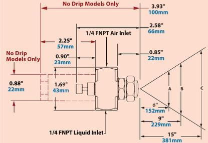
No Drip Only Dimensions in Red See page 69 for No Drip Atomizing Nozzles
