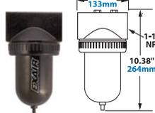
EXAIR's Filter Separators remove water, dirt and rust from your compressed air system. They prevent these contaminants from plugging or damaging the compressed air products. A Filter Separator should be installed prior to an oil removal filter, pressure regulator or valve.
