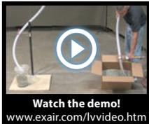
EXAIR's compressed air operated Line Vac connects to standard hose or tube to create a powerful in-line conveyor. The compact design features large throat diameters for maximum throughput capability. Eleven sizes in aluminum and ten in stainless steel are suited to a wide variety of transfer applications.
