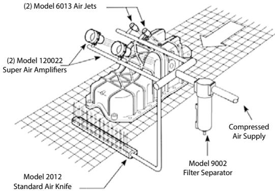
**The Problem:** A newly designed transmission pan presented a myriad of cleaning problems for the die-caster. Because the configuration included channels and blind holes as well as smooth surfaces, a “shaped” air pattern was required for proper cleaning. No single blowoff product would fit the need. An assortment of open copper tubes and drilled pipes was considered, but was rejected as too noisy and expensive
