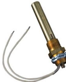
The adjustable thermostat is factory set at 95°F (35°C). It will normally hold  $\pm 2^\circ\text{F}$  (1°C) of the desired temperature setting. It is rated 24V-240V AC or DC, 50/60Hz and is UL Recognized, CSA Certified.
