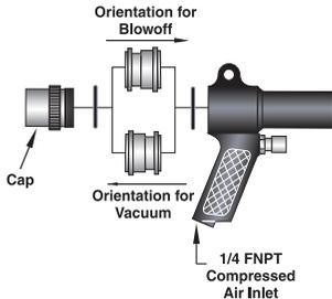
Reverse the direction of the nozzle insert to change from vacuum to blowoff.
