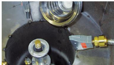
2" Super Air Nozzles blow off metal parts as they are lifted through a vacuum chamber.
