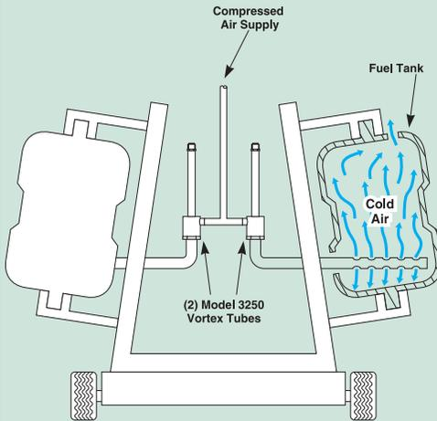
**The Problem:** Automobile fuel tanks are blow molded, then clamped to a fixture to prevent distortion during the cooling cycle. The cooling time of over 3 minutes required for each tank created a bottleneck in the production process.
