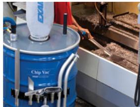
110 Gallon Chip Vac offers maximum capacity cleanup on a large machining operation.
