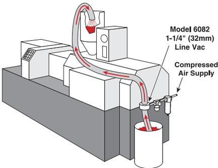
**The Problem:** Injection molding machines transform plastic pellets into various plastic products. The pellets are gravity fed from a hopper on top of the machine. The “bucket and ladder” method of replenishing the hopper was inefficient and expensive.
