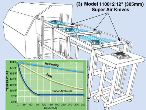
**Comment:** The laminar airflow of the Super Air Knives was the key to success in this application. Fan cooling could only provide random spikes of air at moderate velocities. **The uniform sheet of air from the Super Air Knife quietly swept the heat away within the first 2' (610mm) of the conveyor.** Low air consumption and the compact size of the Super Air Knife were an added bonus.
