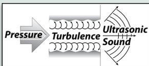
Ultrasonic sound is a range of sound that is above human hearing capacity. Most people can hear frequencies from 20 Hz to 20 kHz. Sound from 20 kHz to 100 kHz can not be heard and is called "ultrasonic". The Model 9061 Ultrasonic Leak Detector converts ultrasonic sound emissions to a range that is audible to people. (The sound generated by the ULD is 32 times lower in frequency than the sound that is received.)
