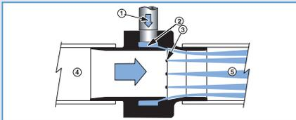
Compressed air flows through the inlet (1) into an annular plenum chamber (2). It is then injected into the throat (3). These jets of air create a vacuum at the intake (4) which draws material in and accelerates it through the unit (5) for conveying over long vertical or horizontal distances.
