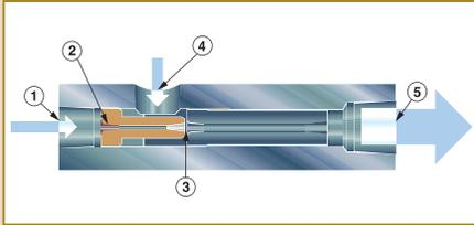
Compressed air flows through the inlet (1), then through a single directed nozzle (2). As the airstream exhausts, it expands and increases in velocity prior to passing through the venturi (3). A vacuum inlet tangential to the primary airflow (4) is located at the suction point between the orifice and the venturi. The airflow that is drawn through the vacuum inlet mixes with the primary airstream, then exhausts on the opposite end (5).
