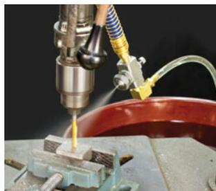
A Model SR1010SS is used to supply a cooling mist for a drilling operation.
