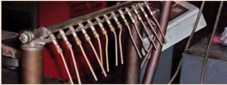
Turbulent compressed air blasts straight out of the pipe or tube. It not only wastes huge amounts of compressed air but also violates OSHA noise and dead ended pressure requirements.
