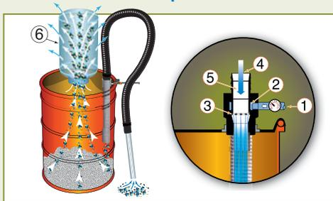
Compressed air, normally 80-100 PSIG (5.5 - 6.9 BAR), flows through the inlet (1) into an annular plenum chamber (2). It is then injected into the throat through directed nozzles (3). These jets of air create a vacuum at the intake (4) which draws material in, accelerates it through the unit (5), and directs it to the bottom of the drum. The airflow exhausts through the port in the drum lid. Airborne particles are trapped by the filter bag (6).
