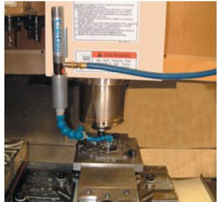
The Model 5315 Cold Gun cools a two flute 3/8" carbide cutter on a CNC, increasing tool life by 50%.
