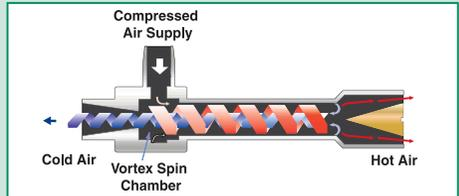
The Mini Cooler incorporates a vortex tube to convert a small amount of compressed air into two low pressure streams, one moving within the other in opposite directions (see page 139). The two airstreams exchange heat, producing cold air from one end of the tube and hot air from the other. A flexible hose directs the cold airstream at the surface to be cooled.
