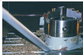
The Chip Vac removes abrasive stainless steel chips from a CNC.
