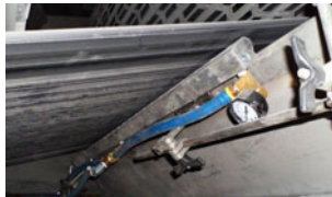
A Model 110048PK1 48" (1219mm) Super Air Knife with Plumbing Kit installed uses EXAIR's Universal Air Knife Mounting System to maintain proper position for removing dust on a conveyor belt and eliminate carryover accumulation.
