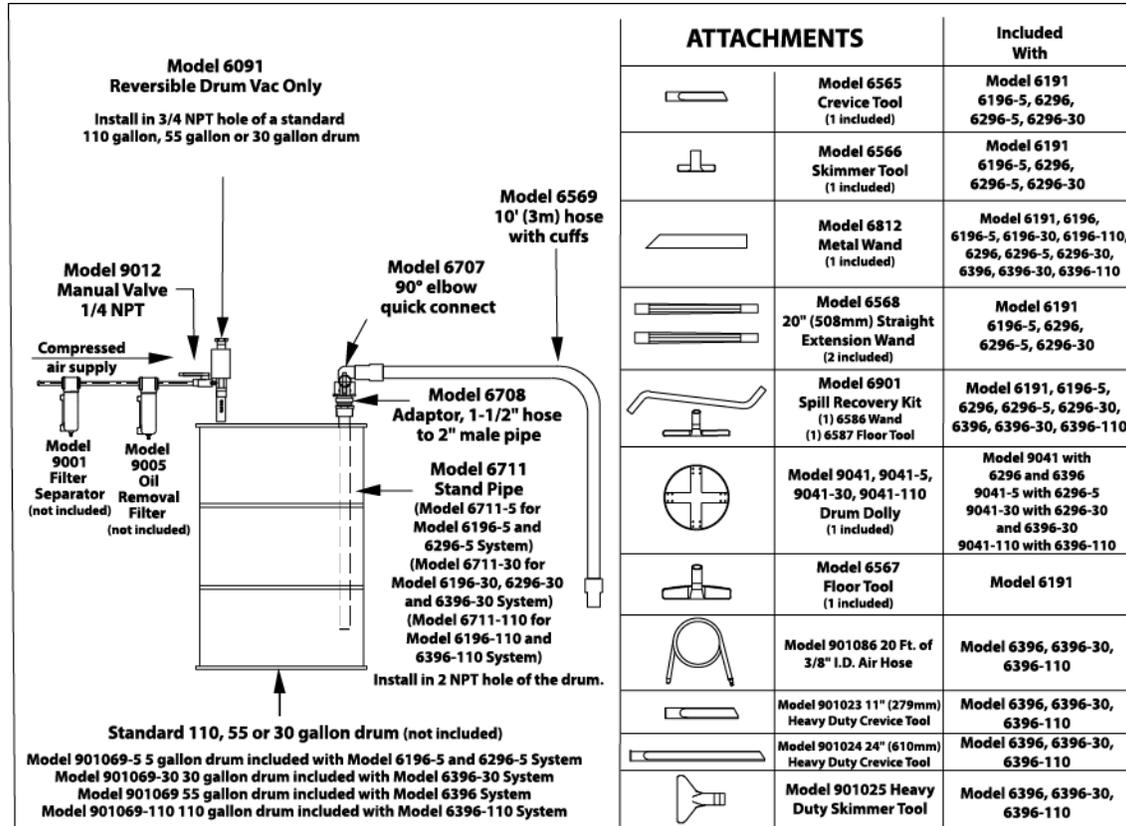
Note: The Reversible Drum Vac System must be used with a closed head steel drum with a minimum wall thickness of 1.5mm (16 gauge) and in good condition.
