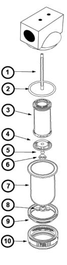
If oil appears downstream: 1) check downstream air lines to be sure that they are free of residual oil; 2) check to see that the filter element and O-ring are in good condition and installed properly.
